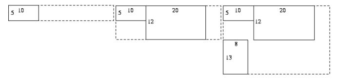
The final dimensions of the resulting window are  $30 \times 25$ , since the width of the first row is 10+20 = 30 and the combined height of the first and second rows is 12+13 = 25.
