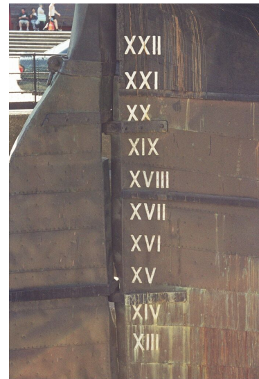
Roman numerals on stern of the ship Cutty Sark showing draught in feet. The numbers range from 13 to 22, from bottom to top. (CC BY-SA 3.0)
