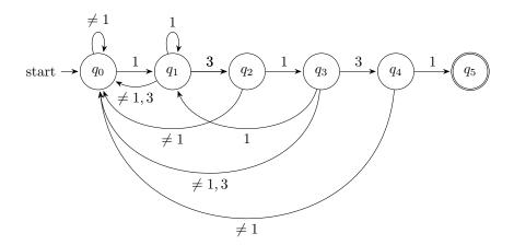
We can simply take each of those six automata states as a DP dimension to track how many prefixes are in each state, using the automata itself to compute the next state:
