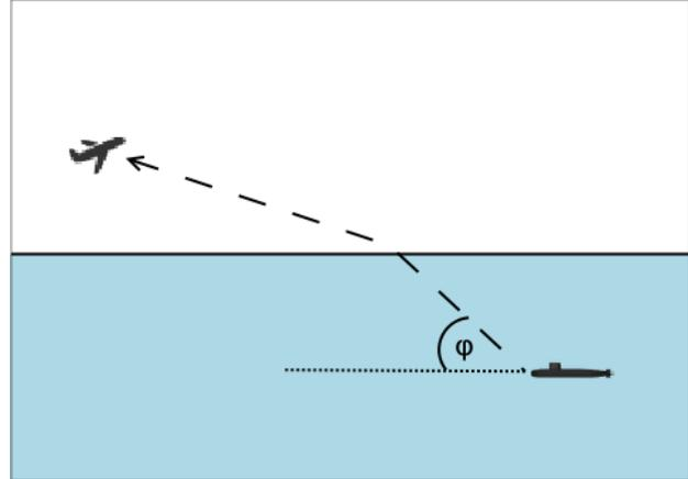
When the laser passes from the sea into the air, it is refracted (its path is bent). The refraction is described by Snell's law, which says that light approaching the horizontal surface at an angle  $\theta_1$ , measured from the vertical, will leave at an angle  $\theta_2$ , given by the formula
