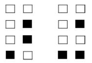
Figure 1. Watch face showing a 24-hour time of 1615.
