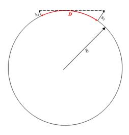
**Figure 1.** "Line of Sight" between source and receiver on an exoplanet's surface. D is the curved surface distance on the exoplanet.  $h_1$  and  $h_2$  are perpendicular to the local surface.
