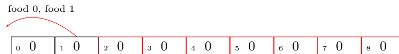
Figure 6.5: evaluation of entry 1. Both food types go off the end of the array, so there is no solution
